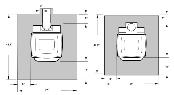
Figure 10. Floor Protection minimum dimensions, CAN. Rear Exit .
