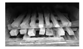
Figure 26. Arrange remaining fuel start-up pieces
