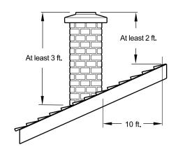
Figure 4. Chimney Height Requirement.
