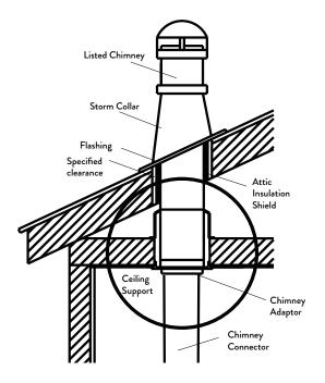
Figure 8. Prefabricated Listed Type HT Chimney.
