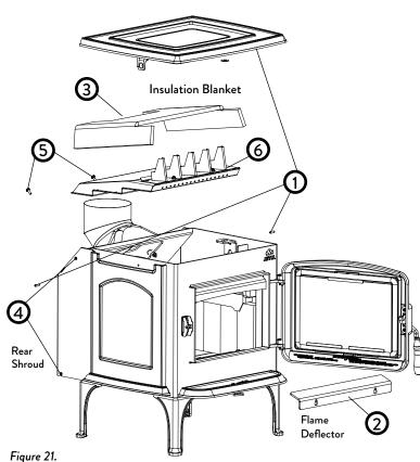
Secondary Baffle removal.
