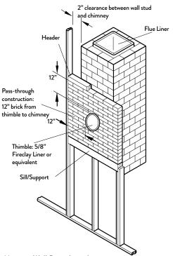
Figure 5. Masonry Wall Pass-through.
