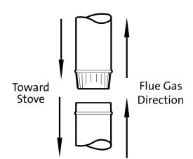
Figure 3. Chimney connector orientation.
