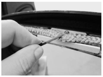
Figure 20. Loosen the glass clips.
