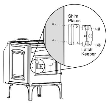
Figure 18. Latch adjustment.
