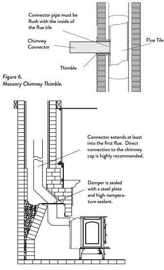
Figure 7. Hearthmount Installation.
