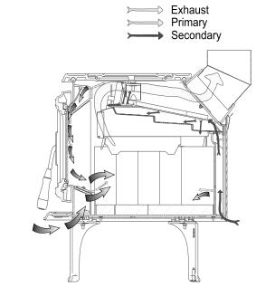
Figure 15. Combustion air paths
