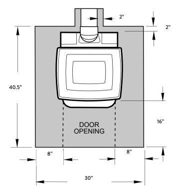
Figure 9. Floor Protection minimum dimensions, U.S. Rear Exit.
