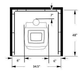
Figure 12. Alcove with Wall Protection.
