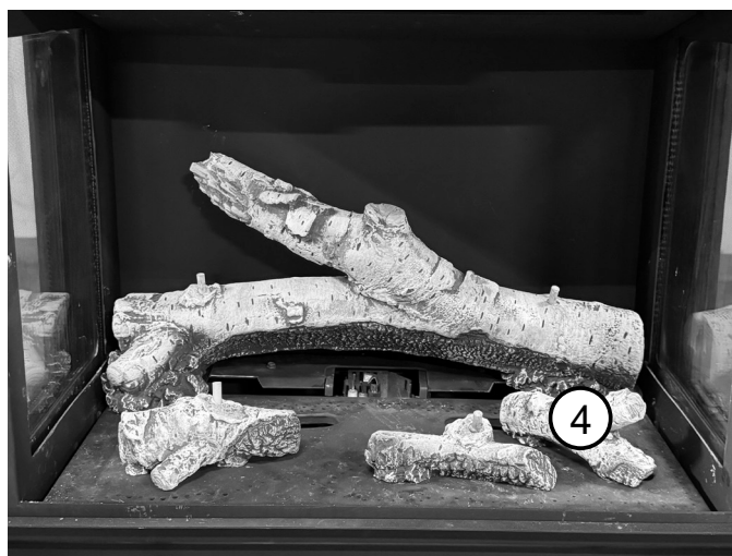
Figure 11.10. Place the #4 Right Lower Log on the two pins on the right side of the burner.
