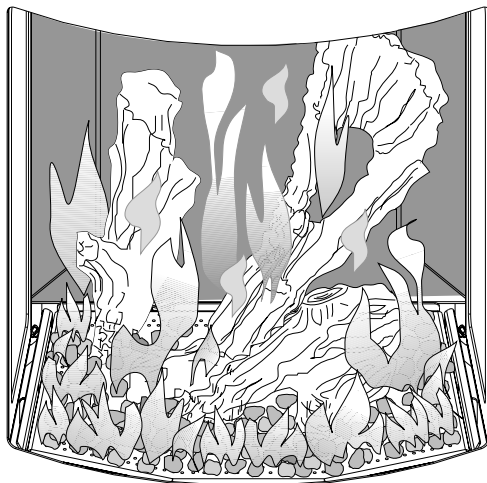
Figure 7.18. Proper flame picture -Traditional Logs.
