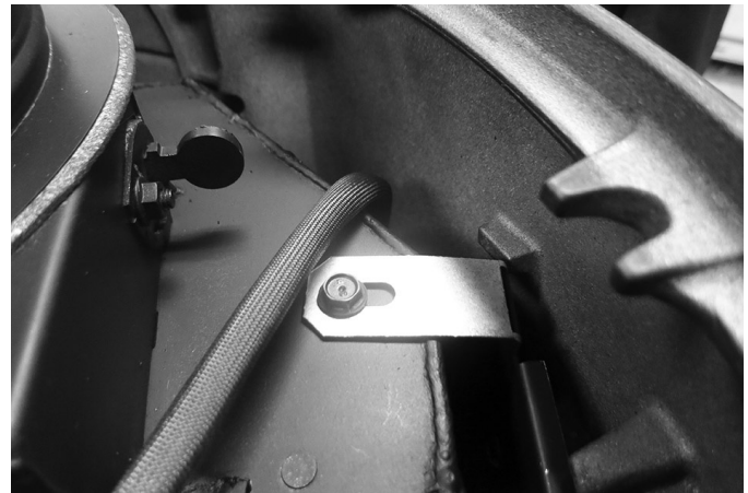
Figure 16.2. Remove the firebox-to-side plate bolt.
