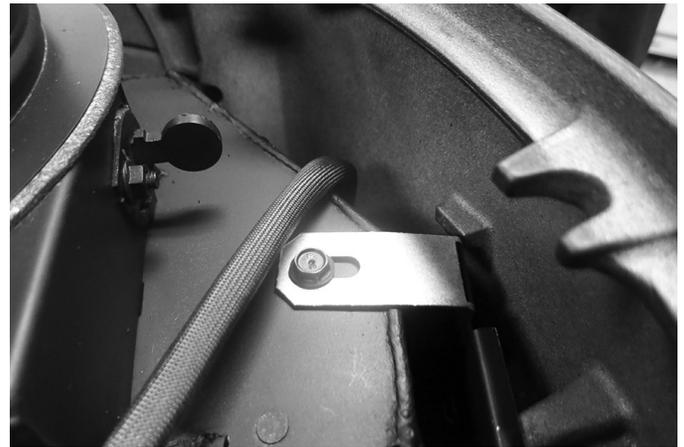
Figure 16.2. Remove the firebox-to-side plate bolt.
