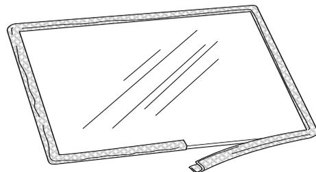
Figure 46. Wrap the gasket around the glass panel.
