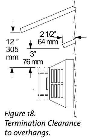
Figure 18. Termination Clearance to overhangs.
