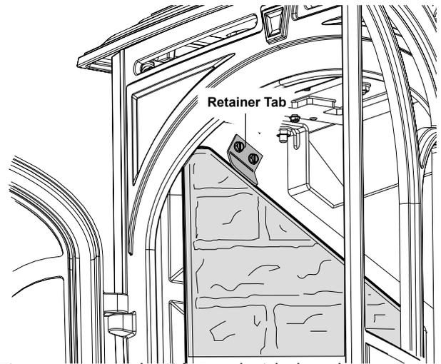
Figure 31. Secure the Side Panel with the tab.
