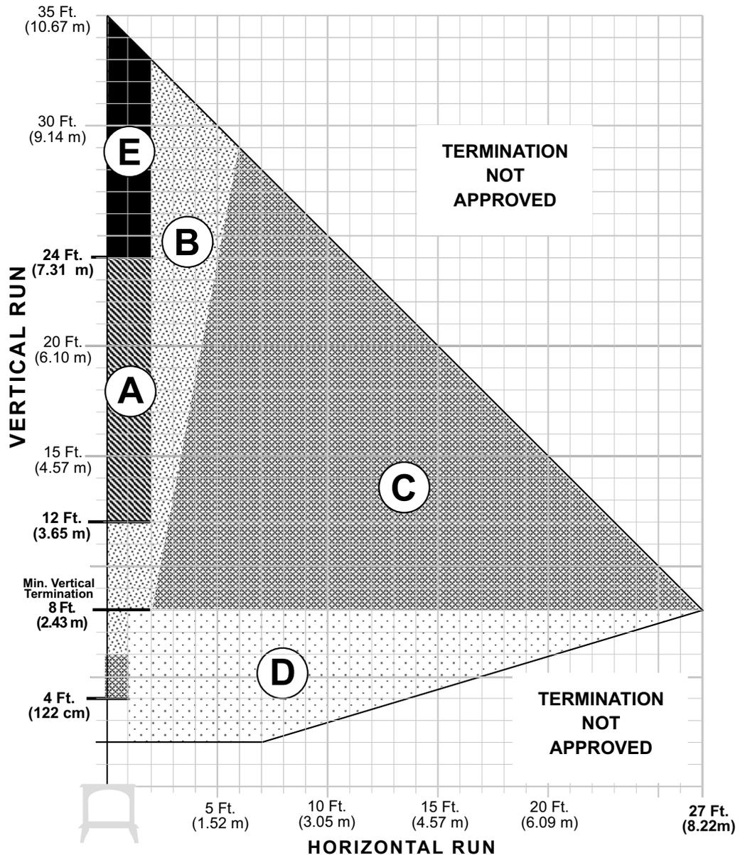
Figure 9. Vent Termination Matrix - NG / LP
