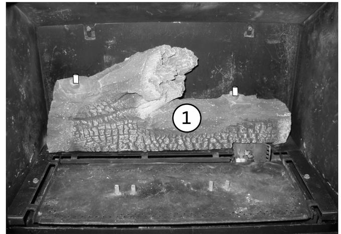
Figure 33. Locate the Rear Log over the two pins on the back shelf of the burner skirt.
