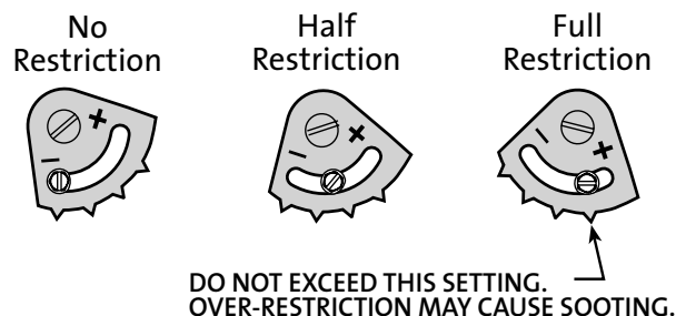
Figure 15. Exhaust Restrictor settings
