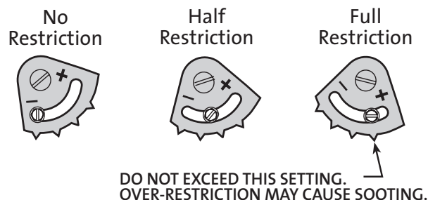
Figure 15. Exhaust Restrictor settings
