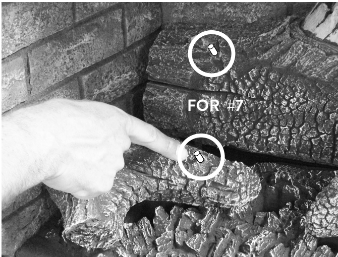
Figure 47. #7 Log: Engage the underside holes with the pins in Log #1 and Log #2.
