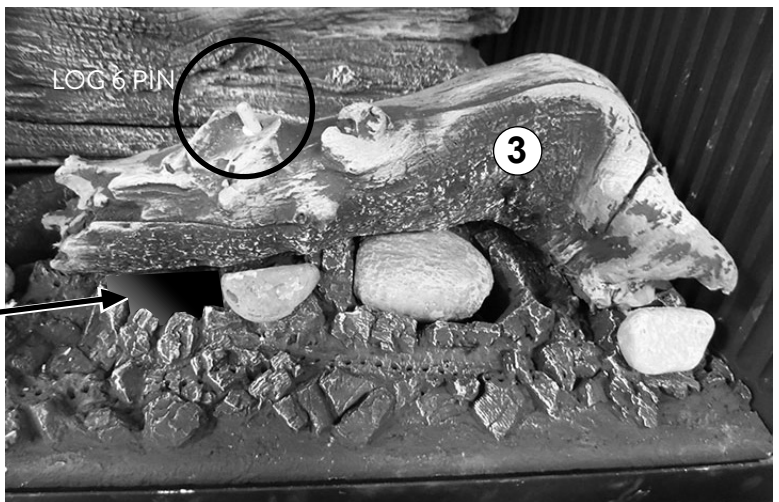
Figure 60. Orient Log 3 behind the rocks, engaging the right end with the large slot in the burner base.
