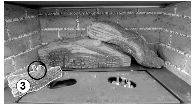
Figure 7.14. Engage the holes in the underside of Left Burner Log #3 with the matching pins on the burner plate shown in fig. 7.13.
