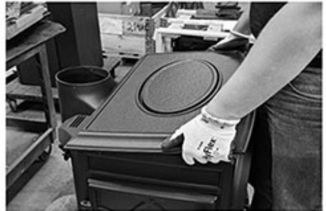
Fig. 21. Remove the top plate from stove.
