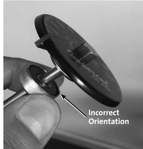
Fig. 13c. Remove magnet from current orientation
