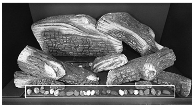
Figure 7.20 Position Burner Embers in row on burner. Be careful to avoid obstructing the pilot and burner carry-over ports shown in fig. 7.21.
