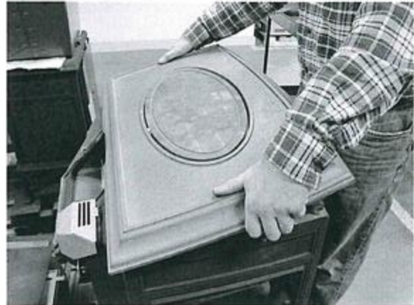
Fig. 20. Pull top plate forward to release stud from back plate.
