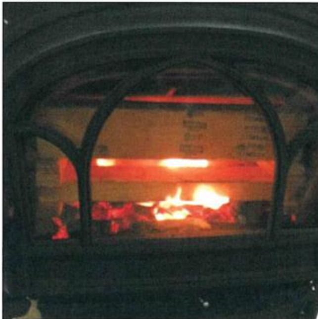
Typical Test Fuel Loaded in Test Stove
