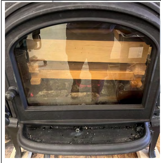
Test Fuel Loaded in Stove
