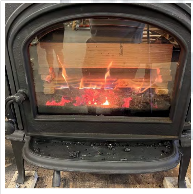
Test Fuel Loaded in Stove
