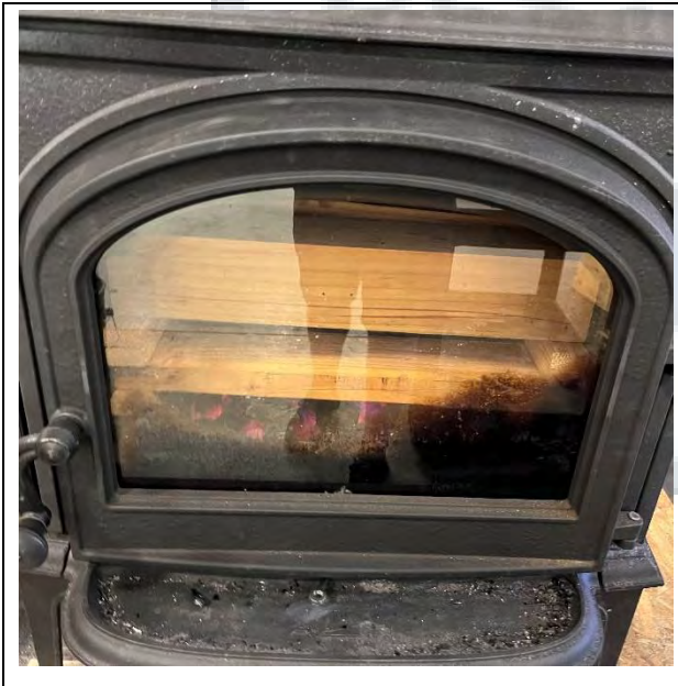
Test Fuel Loaded in Stove
