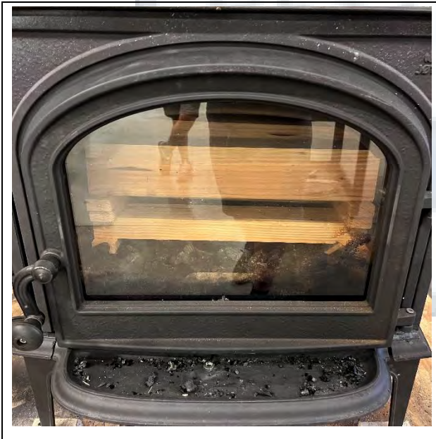
Test Fuel Loaded in Stove
